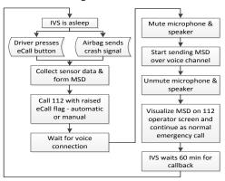
Fig. 2 Normal eCall workflow
