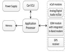
Fig.3 Basic structure of a real-life IVS device
