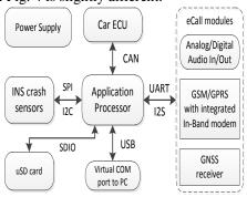
Fig.4 Structure of TUS's IVS prototype
